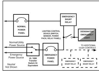
**Wiring Diagram #1:** A dedicated switch or line voltage dimmer controls emergency lighting in a space. Upon loss of normal power, the emergency lighting comes on at full brightness regardless of switch or dimmer position. NOTE: LUT-SHUNT-FM is not for use with 0-10V DIMMER. Use LUT-SHUNT-D-FM.
