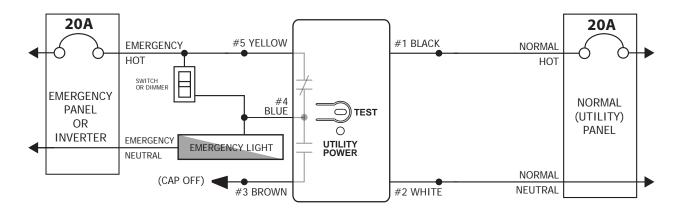
**Wiring Diagram #2:** For use with Lutron Vive integral fixture controls and DALI drivers with self powered DALI link, such as Philips® SR XI040C110V054VPT1 and XI075C200V054VPT1 and Osram ® Dexal (tm) OTi50/120-277/1A4 DX L and OTi30/120-277/1A0 DX L
