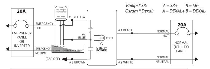
**Wiring Diagram #3:** For use with Lutron Vive integral fixture controls and EcoSystem drivers without self powered DALI link, such as Lutron LDE1, LDE5, L3D, and L3D0
