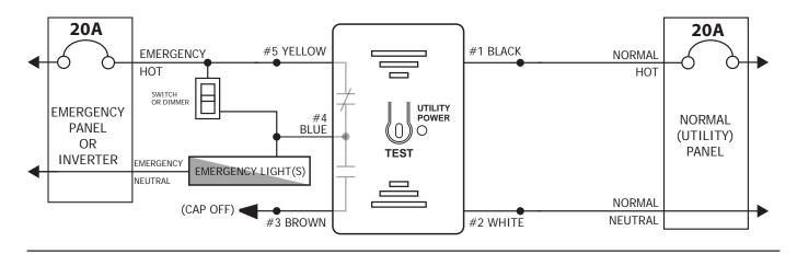
**Wiring Diagram #2:** Slave Relay Application - LUT-SHUNT can be used to switch an auxiliary load (similar to a lighting contactor) in case your switch is rated <20A or to switch a 277V load from a 120V switch.
