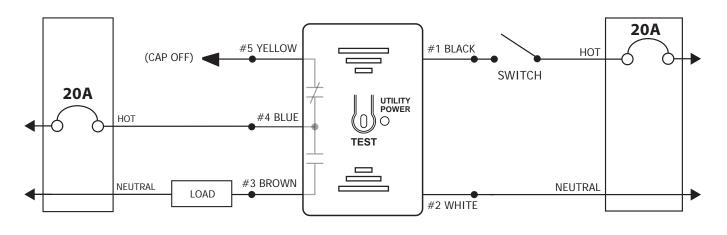
**Wiring Diagram #3:** *EcoSystem - LUT-SHUNT can be used to interrupt an EcoSystem signal and drive emergency lighting to full brightness upon loss of the local normal lighting circuit.*
