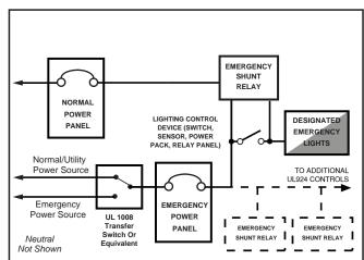
**Wiring Diagram #1:** A dedicated switch or line voltage dimmer controls emergency lighting in a space. Upon loss of normal power, the emergency lighting comes on at full brightness regardless of switch or dimmer position. NOTE: LUT-SHUNT is not for use with 0-10V DIMMER. Use LUT-SHUNT-D or LUT-ALCR-D
