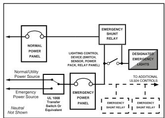
**Wiring Diagram #1:** A dedicated dimmer controls emergency lighting in a space. Upon loss of normal power, the emergency lighting comes on at full brightness regardless of dimmer position.
