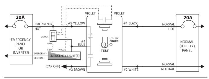
Wiring Diagram #2: Wireless controller with electrically held relay, such as Vive.
