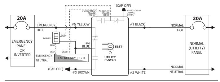
Wiring Diagram #2: Wireless controller (CAP OFF) 20A 20A #5 YELLOW #1 BLACK EMERGENCY NORMAL HOT HOT OLET **EMERGENCY LIGHT** #4 BLUE **NORMAL** GRAY **TEST** (UTILITY) **PANEL** 0 UTILITY POWER **EMERGENCY** NEUTRAL NORMAL **EMERGENCY** NEUTRAL #3 BROWN #2 WHITE **PANEL**
