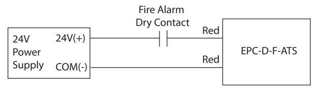
Note: EPC-D-F-ATS red wires are polarity independent
