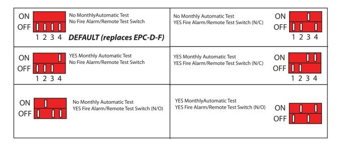
Monthly Automatic Test feature will test EPC-D-F-ATS for 40 seconds every 25 days and record result on microprocessor. Test results may be played back by holding test button for 3 seconds. Once green LED flashes once, release test button. Every green flash signals a passed test, every red flash signals a failed test. Annual testing for 90 minutes is still required and recommended.
