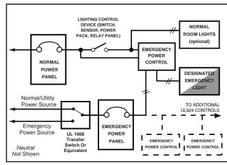
**Wiring Diagram #1 (Suggested):** A dimmer (fed by normal power) controls emergency lighting in a space. Upon loss of normal power, the emergency lighting comes on at full brightness regardless of dimmer position.
