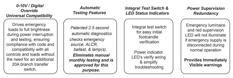
LVS Emergency Power Controls are tested, approved, and listed by Underwriters Laboratories under UL 924 standards for designated emergency light fixture controls. They meet and exceed all pertinent code requirements from NEC, NFPA, OSHA, and life safety codes, in addition to major local codes. All model LUT-ALCR-D-HV-347V are tested burned in during production.
